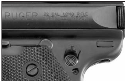
Figure 5. Safety in the “off” or “fire” (F) position. Safety is all the way down .
