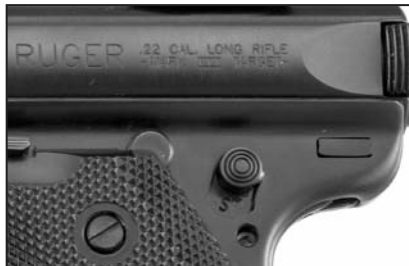
Figure 6. Safety in the “on” or “safe” (S) position. Safety is all the way up .
