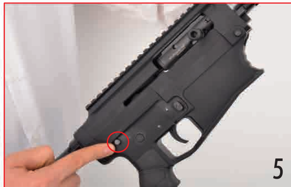
5) Push the other detaching pin and pull from the other side until it sets
