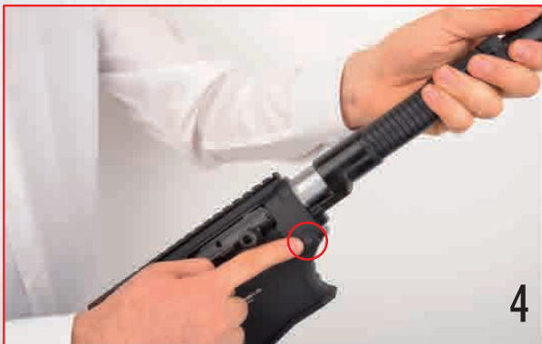
4) Push the detaching pin and pull from the other side until it sets
