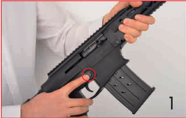
1) Remove the magazine
