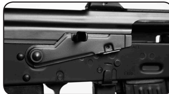
Picture #5 BOLT CATCH - Safety engaged! Bolt is exposed, blocked and the trigger is blocked from full travel. FIRE DISABLED!
