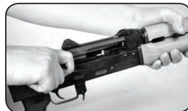
Picture #7 Pull Bolt charging handle all the way back to expose the chamber
