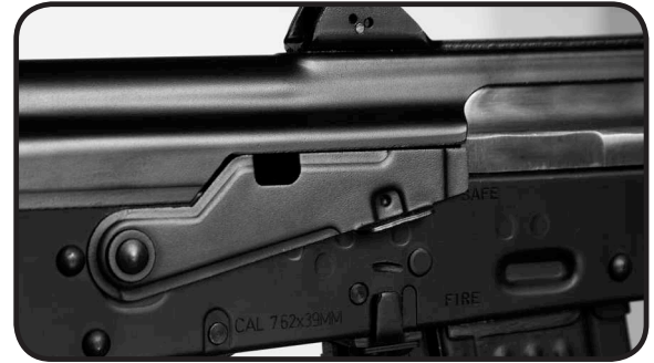
Picture #2 SAFETY ENGAGED! Bolt is covered and the trigger is blocked from full travel. FIRE DISABLED!
