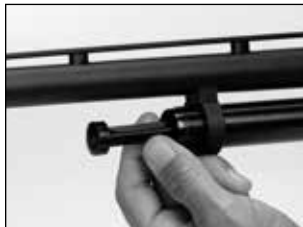
Pull the three-shot adaptor out of the magazine tube with your fingers.
