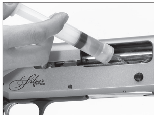
Occasionally place a drop of light gun oil on the rails inside the receiver.
