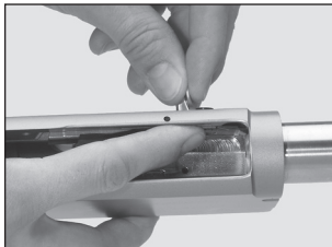
Pull outward to remove the bolt handle (12 gauge).
