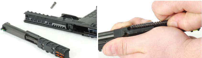
Slide assembly removed from grip assembly and compressing the recoil springs
