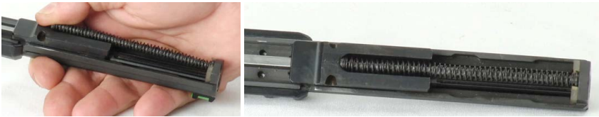
Snapping the captive recoil springs in place
