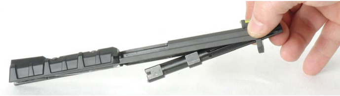
Barrel now can be removed from the slide
