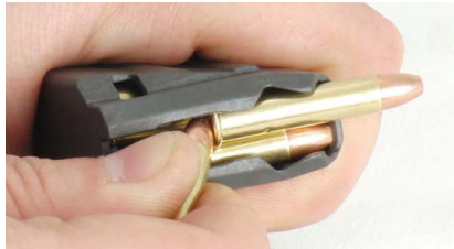
Unloading the magazine by pushing rounds forward
