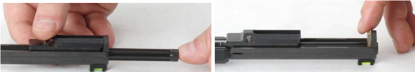
Dropping the barrel block in, sliding it back, and inserting the buffer
