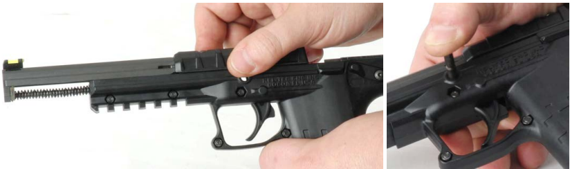
Sliding the upper assembly back on the grip and inserting the assembly pin
