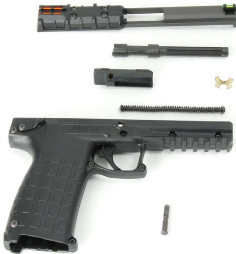
Fully Field Stripped
