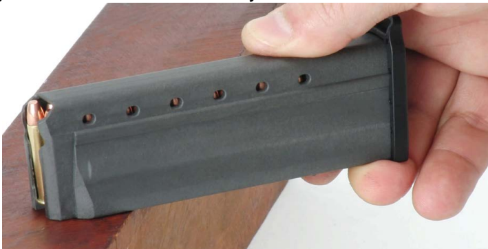
Tapping the back of the magazine on a flat surface to seat rounds and ease loading
