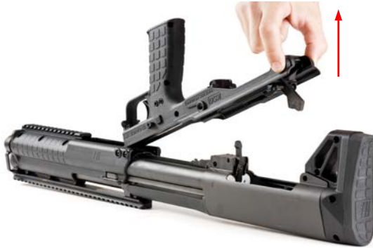
Figure D-3: Lift Grip Assembly Directly Upwards
