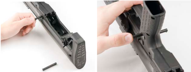
Figure D-2: Place Rear Assembly Pins in Retaining Holes
