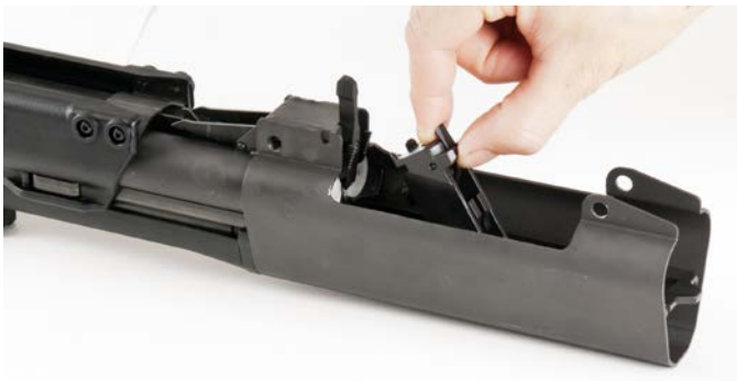
Figure D-5: Remove Bolt from Receiver
