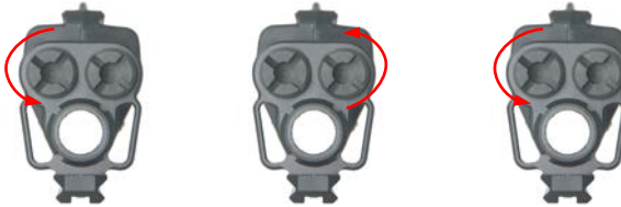
Figure D-6: Unscrew Magazine Bolts with Alternating 1/2 Turns
