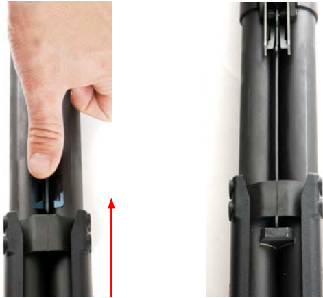
Figure E-3: Slide Forend over CTG Stop Actuator to Secure Assemblies
