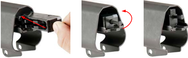
Figure E-5: Insert Bolt onto Bolt Carrier Sideways and Rotate 90°
