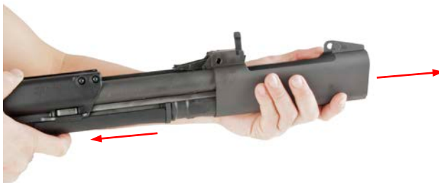
Figure D-9: Pull Barrel Assembly Apart from Receiver Assembly
