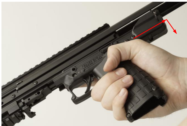
Figure D-2: Slide grip straight back, then pull away
