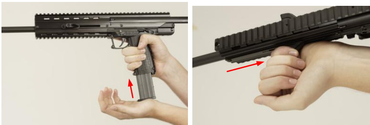
Figure C-4: Slapping the base of the full magazine and pulling operating handle back to chamber a round
