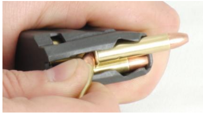
Figure C-6: Unloading the magazine by pushing rounds forward
