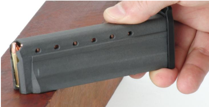
Figure C-3: Tapping the back of the magazine on a flat surface to seat rounds and ease loading
