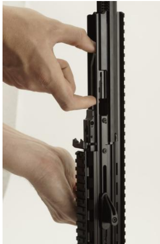
Figure D-3: Grip bolt block as shown, after lifting it with the operating handle
