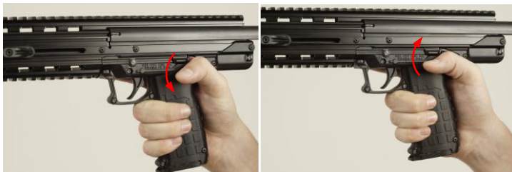
Figure C-5: Sweeping the safety lever down for FIRE, or up for SAFE
